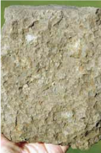
MODERATE CONDITION VS = 1 Soil has many (10–20 percent) fine and medium orange and grey mottles.
